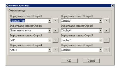
Define tags for respective Output port, then displays connect the Output ports can be easily remembered.
